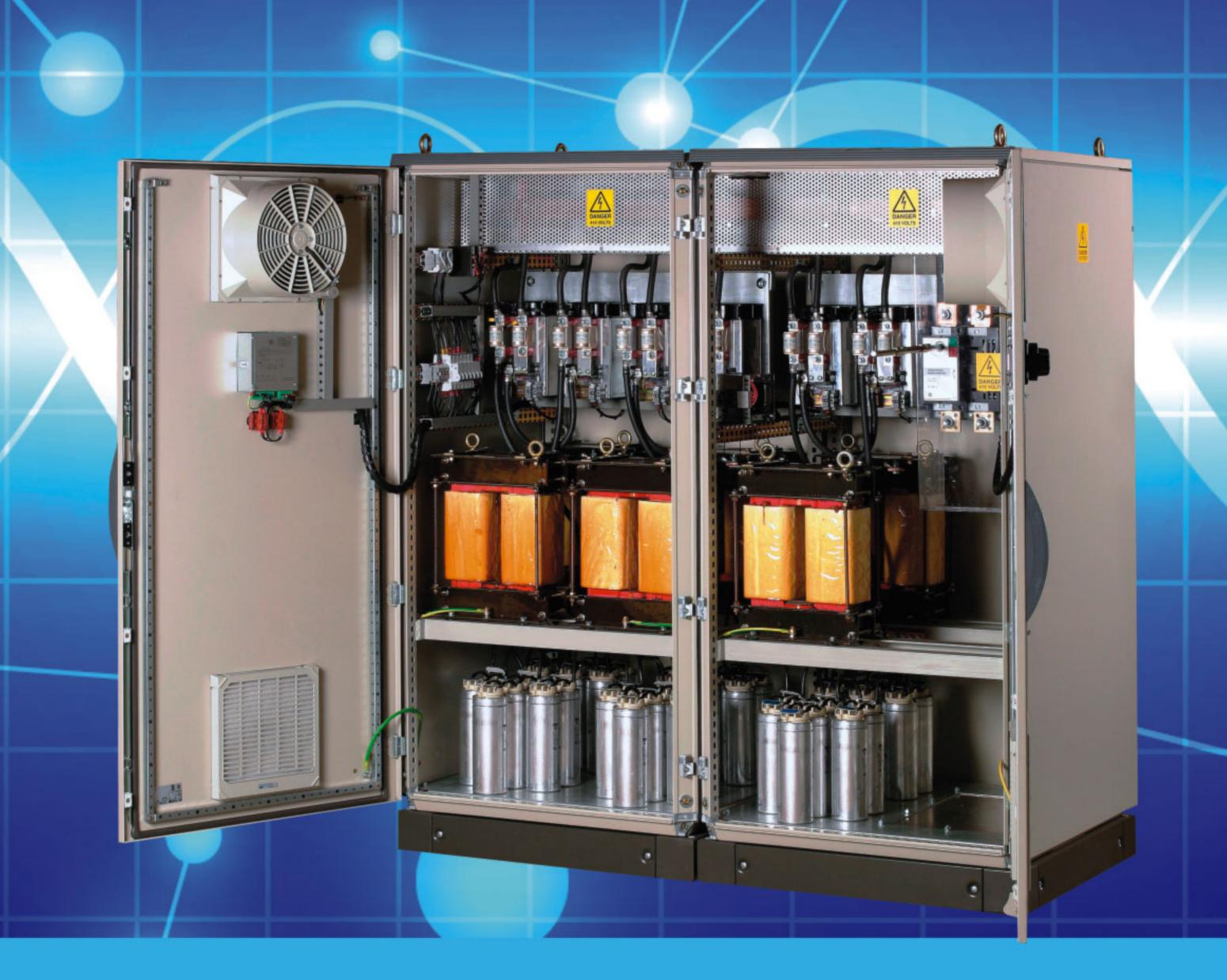
Certain equipment such as drives, inverters, UPS, arc furnaces, transformers, filters and discharge lamps generate harmonics. The harmonics strain the network. Voltage distortion overload cables, cause failures of relays and circuit breakers and disturb many types of equipment such as computers, telephones etc.. Implemented by experienced specialists, the harmonic filtering solutions eliminate most of the power quality problems.
